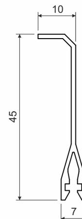
product description: it is used to divide the interior of the trunking, thus allowing a better manipulation with the inserted cables and clarity
